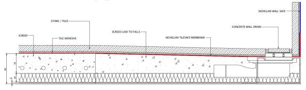
**8.** Once the screed is dry, the area is then ready for the the Novellini floor and wall membrane to be installed.
