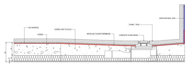
**8.** Once the screed is dry, the area is then ready for the the Novellini floor and wall membrane to be installed.
